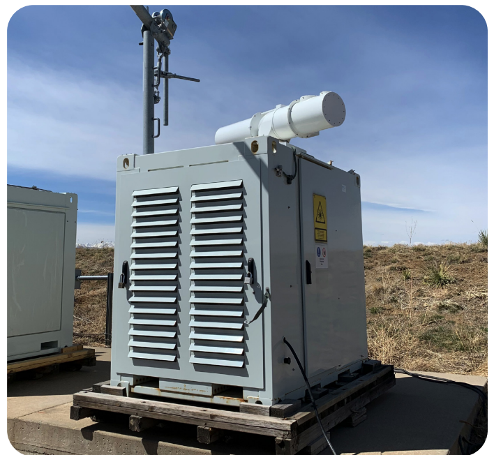
1 of 2 LiDAR machines shortly on its way to be installed in Portland
